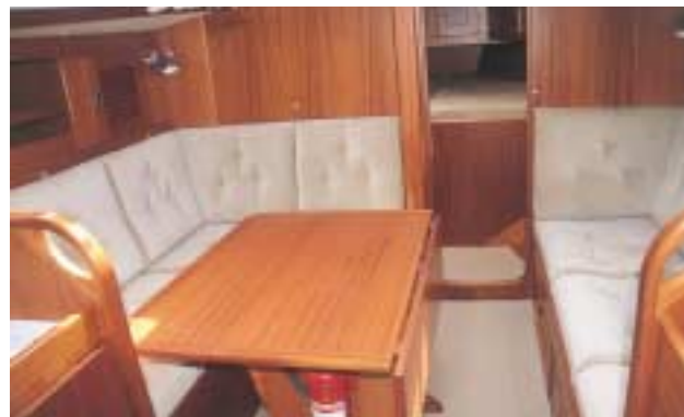
The saloon features an L-shaped settee to port, drop-leaf table and a straight settee/passage berth to starboard.
