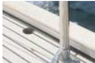
Deck drainage holes are routed through deck to avoid those horrible run-off stains you see on some boats.
