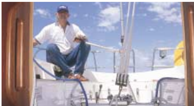
The traveller is in the middle of the cockpit, but low down so it is easy to step over. It is also removable and a table slots in when at anchor.
