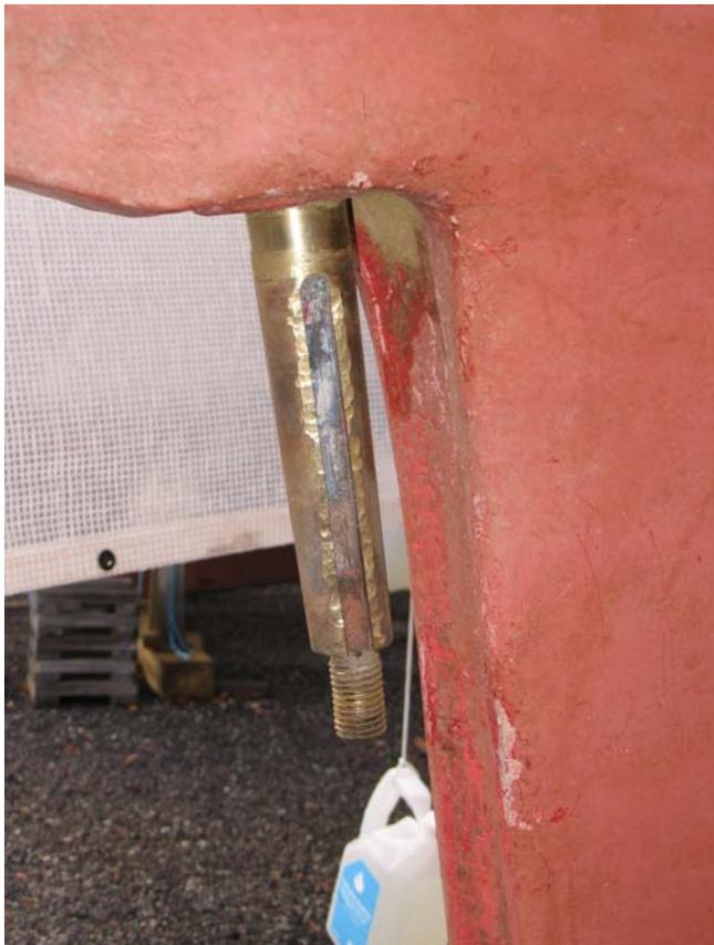
This picture shows what the shaft looked like once the rudder was removed. The shaft is rotated 90 degrees for visibility. As you notice, the shaft surface was a little damaged by the rotating file but I don't think it matters much. The locking key did not want to let go of the axial slot and I could not think of any other way to do it.
