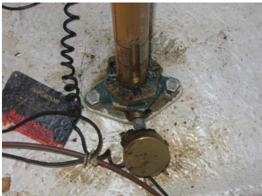
The cavity where the nut is found is covered with fibreglass putty. Use a lightweight hammer and small chisel to remove this. Be careful not to damage the gelcoat surface of the rudder. The upper rudder fitting does not have to be removed so unless the putty covering the tangs that attach it to the rudder is cracked and you want to replace it, you may leave it as is. The cracks will probably also hold
