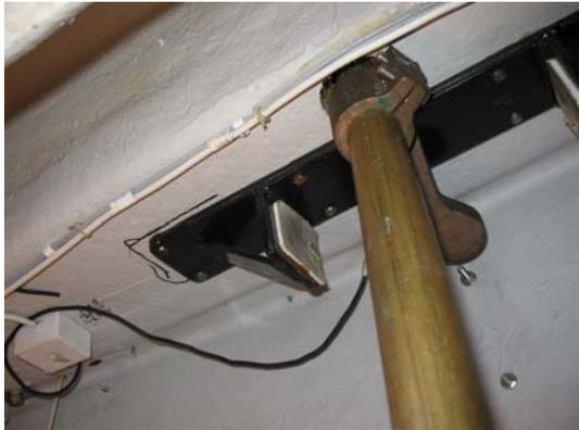
To remove the steering stop (or limiter), loosen the 2 bolts and slide the stop arm downward. There’s a locking key made from steel that prevents the arm from turning on the shaft. You may leave the arm halfway down the shaft.
