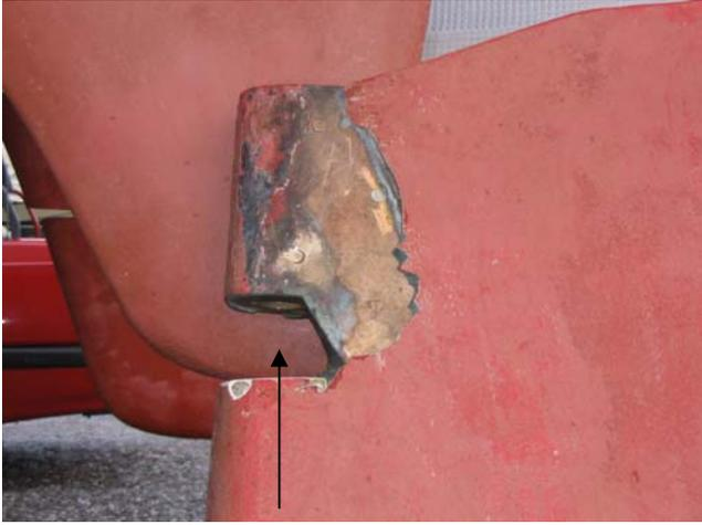
This shows the rudder as removed. Looking closely the vertical slot for the locking key is just visible along the forward edge of the hole.
