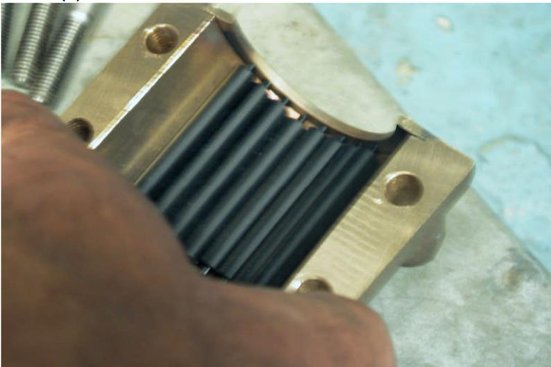
Photos 10, 11 & 12: Thru-Hull Bearing Housing (prior to laminating to hull).
