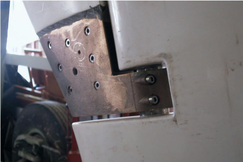
Photos 3 & 4: Skeg Bearing filled, laminated, faired and sanded prior to priming.
