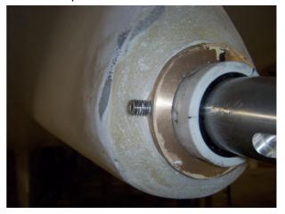
Step 3 : Remove bearing and replace. Pls. note: do not allow propeller shaft to hang in stern tube; risk of damage to gearbox shaft!
