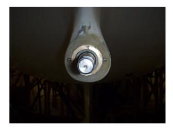
Step 2: Grip the cutlass bearing's composite outer sleeve, rotate and pull to remove.
