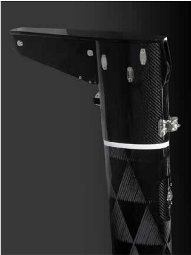
stretch sails with a good service life. The main has an impressive headboard and generous roach, creating a powerful sail with proportions that are only possible with a big carbon crane on the back of the mast head, to allow enough space between the leach and the backstay. This takes the performance of in-mast furling another step forward.
