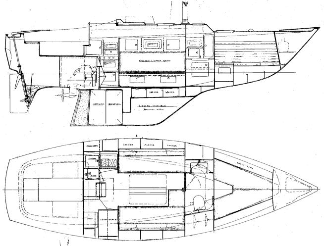
The main cabin is built with fair sized sofa-berths P and SB. The SB side sofa is made as a L-sofa. Behind the swing up backrests is stowage for bedding. The sofas are 6'-6". Bookshelves and lockers outside the sofas. Large table with fold down top panels. Stowroom for bottles etc. in the middle section. The inside of the hull above berths is panelled with mahogany. The ceiling is lined with vinylpanels.
