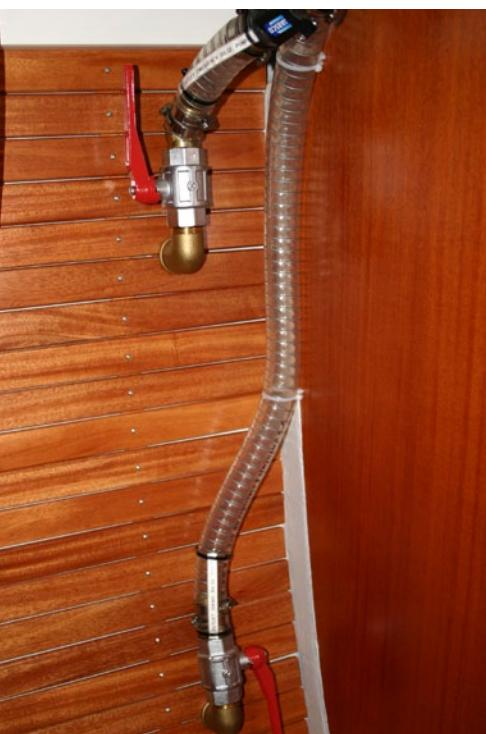
*Easy access to well dimensioned ball valves for through-hull fittings*
