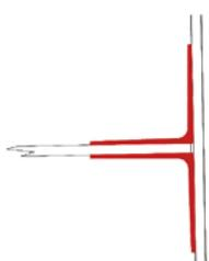
Hull and deck are carefully laminated together on all models. Stanchions are securely mounted, on 37 ft and larger on the top of the cap rail coaming.
