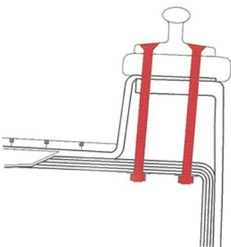
The cleats are firmly secured with four bolts per cleat to the cap rail at the outboard edge of the deck, leaving the inboard area clear so that the crew can move safely about the boat.
