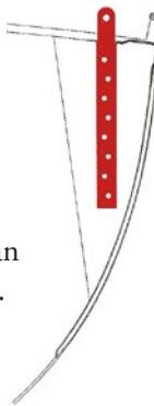
The chain plates are secured to the insulated hull through guides that are inclined so that there is no change of angle throughout their length.
