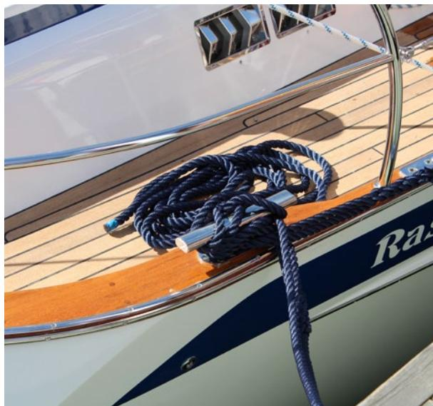
*Sturdy stainless mooring and spring cleats, secured with four bolts each*
