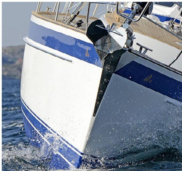
*A sturdy rubbing strake is integral to the hull*
