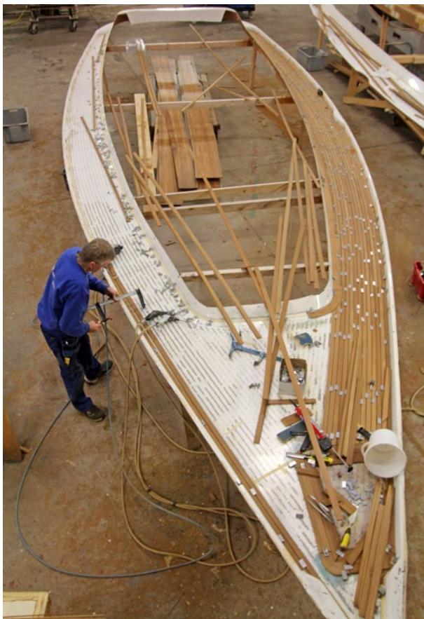
Teak deck, handcrafted on a template outside the boat, 10 mm thick solid wood, completely vacuum glued without screws to the GRP deck for long service life
