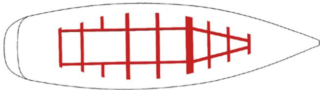
The GRP hull is reinforced with a grid structure at floor level to give it increased stiffness. The grid part under the mast support even has a steel beam moulded into the GRP grid.
