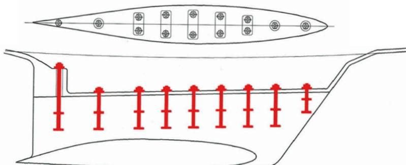
The keel is attached to the hull by stainless steel bolts that are highly resistant to corrosion. Keel material is cast lead to enable the size for a given weight to be kept moderate, so improving the boat's performance. Lead is also softer than iron in case of grounding, and lead cannot rust. The keel is attached to a deep bilge, this also improves the strength.
