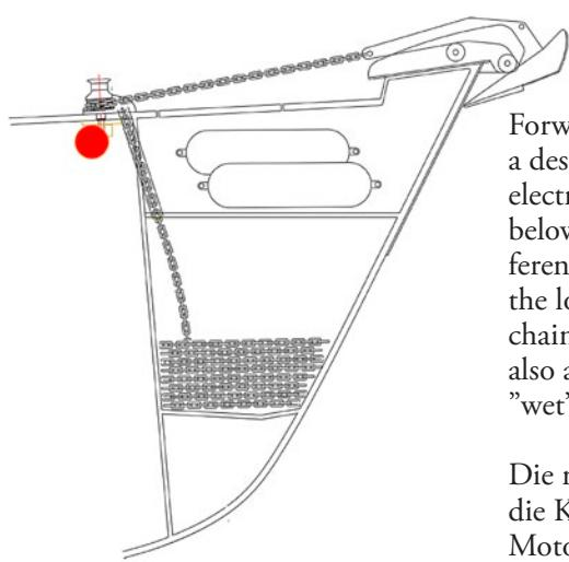
Forward, the chain locker is arranged for self stowing – a design arrangement introduced in 1978 – while the electric windlass has its motor mounted in a dry area below deck to avoid condensation. This height difference makes the chain self-stowing. The opening to the locker is asymmetric to give good access even if the chain is moving. On boats of 34 ft and above there is also a shelf (if electric windlass is ordered) for stowing “wet” items such as fenders.
