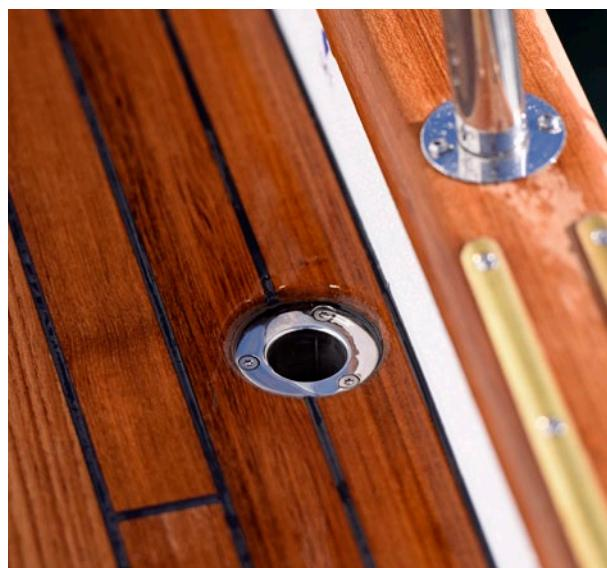
*Deck drains with exits under the waterline, to prevent stains on the hullside*
