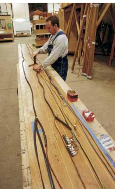
*Wiring is prepared outside the boat*
