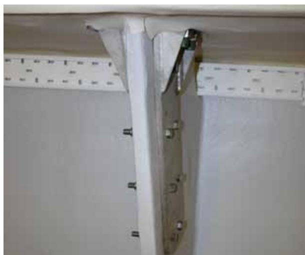
*The support for the rigid stainless chainplates is laminated from both sides to the hull and to the deck to distribute loads*
