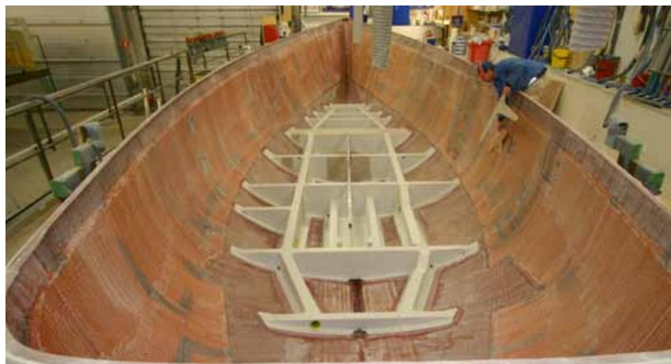
*The grid distributes the loads to the hull*
