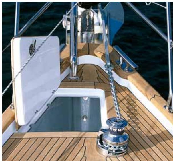
*Asymmetric chain locker opening makes it possible to step to the very front of the boat even if the chain is moving*
