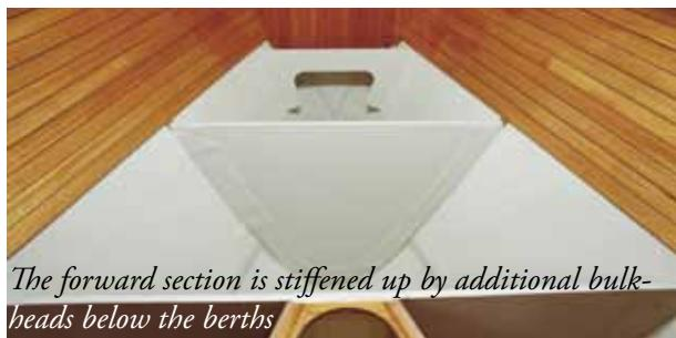
*The forward section is stiffened up by additional bulkheads below the berths*
