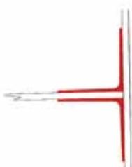
Stanchions are securely mounted using a solid, stainless steel rod recessed into the bulwark and projecting above it, over which the stanchion is slipped and secured (HR 37-62). Hull and deck are carefully laminated together on all models.
