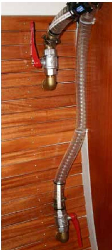
*Easy access to well dimensioned ball valves for through-hull fittings*
