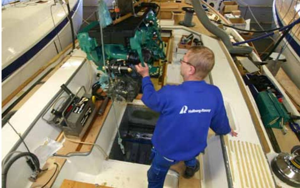
Engine and tanks come in through the normal opening of the boat after that the woodwork is done
