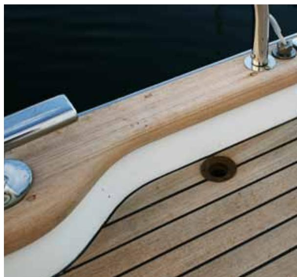
*Deck drains with exits under the waterline, to prevent dirt strips on the hullside*
