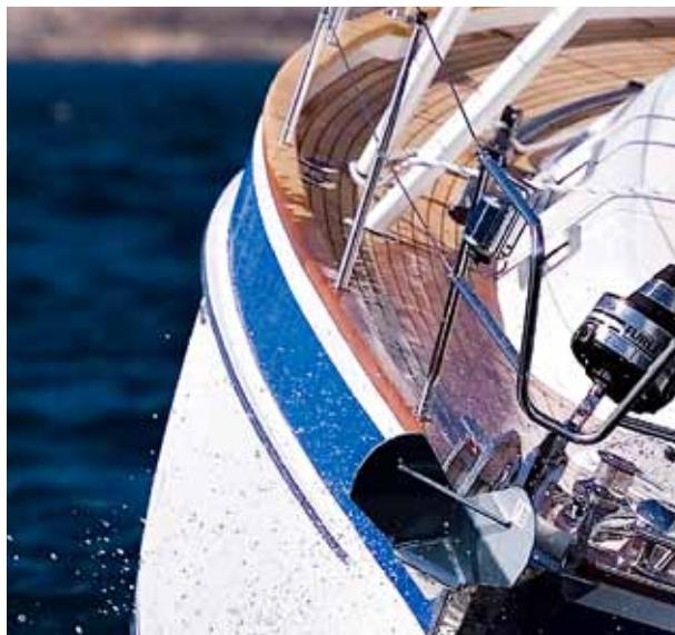
*A sturdy rubbing strake is integrated to the hull*
