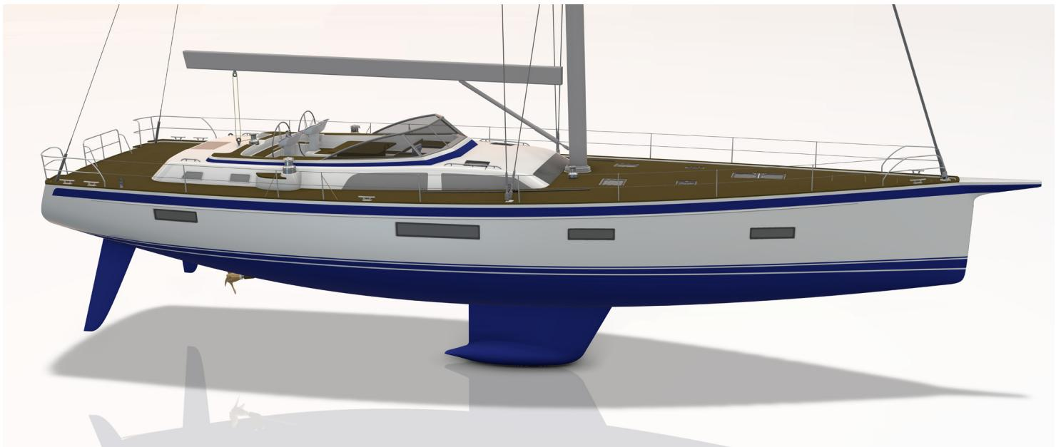
*Hull length 20.96 m / 68' 9", beam 5.89 m, 46,5 t*
